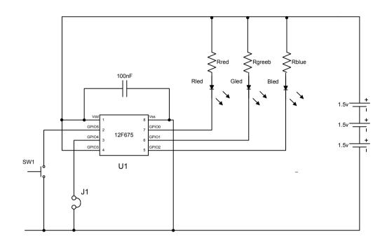
This version of the RGB light uses the same firmware as the version above. Grounding GPIO4 (J1 closed )tells the software to invert the output drives so that they become active low. In this configuration the GPIO pins can sink 25mA each. This circuit should operate from  $3 \times 1.5 \times AA$  batteries
